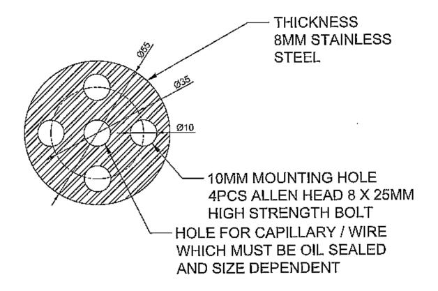
NOTE: 1. FLANGE IS FOR OIL SEALING PURPOSE
